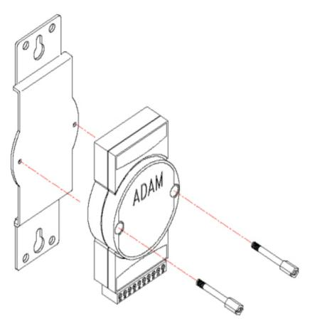
Figure 3.2: Fix Module on theBracket
