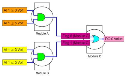
Figure 7.16: Distributed Logic Cascade
