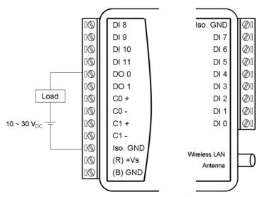
Figure 4.28: ADAM-6051W Digital Output Wiring
