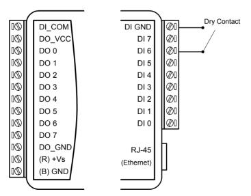
Figure 4.17: ADAM-6052 DI (Dry Contact) Wiring
