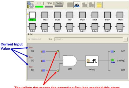
The yellow dot means the execution flow has reached this stage Figure 7.21: Online Monitoring Function
