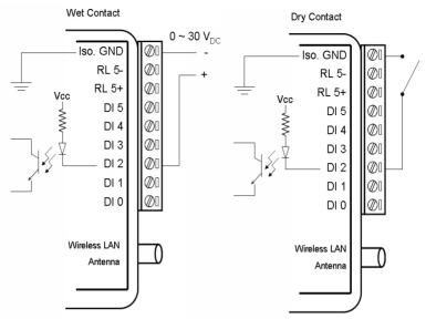
Figure 4.29: ADAM-6060W Digital Input Wiring
