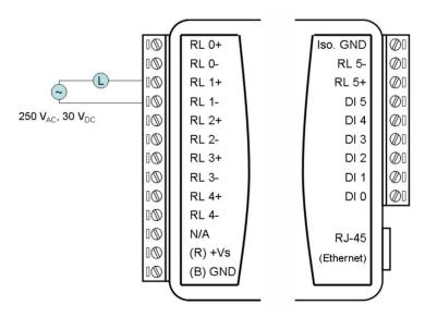
Figure 4.23: ADAM-6066 Relay Output Wiring
