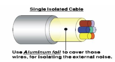
Figure C.9: Single isolated cable
