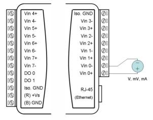
Figure 4.2: ADAM-6017 Analog Input Wiring
