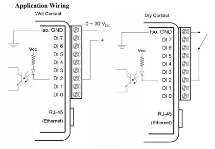
Figure 4.14: ADAM-6051 Digital Input Wiring
