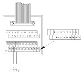
Figure 4.6: ADAM-6018 Thermocouple Input Wiring
