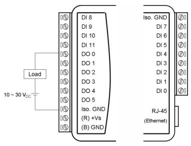
Figure 4.13: ADAM-6050 Digital Output Wiring
