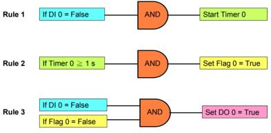
Figure 7.36: GCL Logic for Falling Edge
