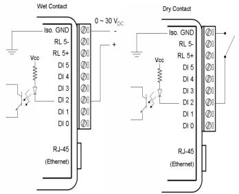
Figure 4.20: ADAM-6060 Digital Input Wiring
