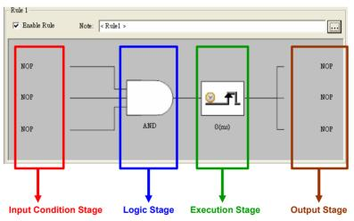
Figure 7.2: Four Stages for One Logic Rule
