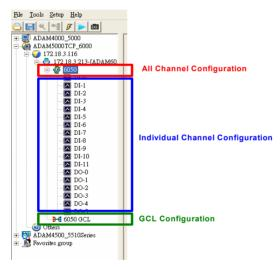
Figure 5.4: Channel & GCL Configuration
