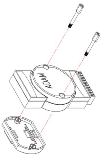
Figure 3.3: Fix Module on the DIN-rail Adapter
