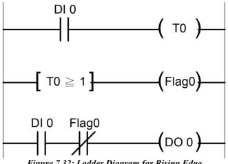
Figure 7.32: Ladder Diagram for Rising Edge
