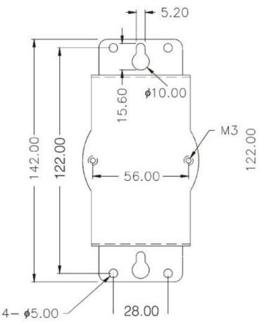
Figure 3.1: Panel Mounting Dimensions
