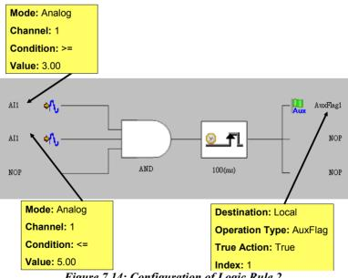
Figure 7.14: Configuration of Logic Rule 2
