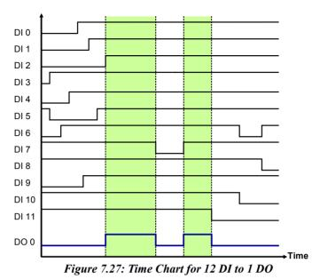
You can simply implement one AND logic operator to achieve this control system. However, since one logic rule only has three inputs, we need
