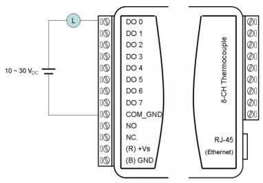
Figure 4.7: ADAM-6018 Digital Output Wiring
