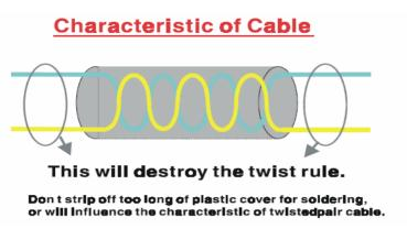
Figure C.12: The characteristic of the cable
