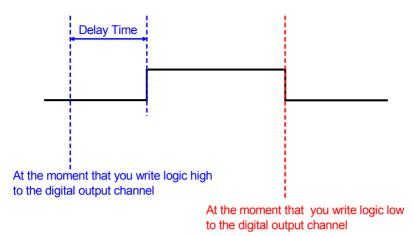
Figure 5.16: Low to High Delay Output Mode
