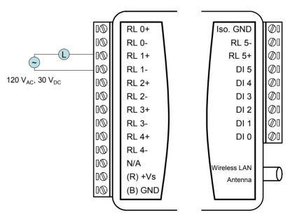
Figure 4.30: ADAM-6060W Relay Output Wiring
