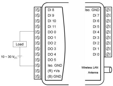
Figure 4.25: ADAM-6050W Digital Output Wiring
