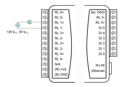
Figure 4.21: ADAM-6060 Relay Output Wiring
