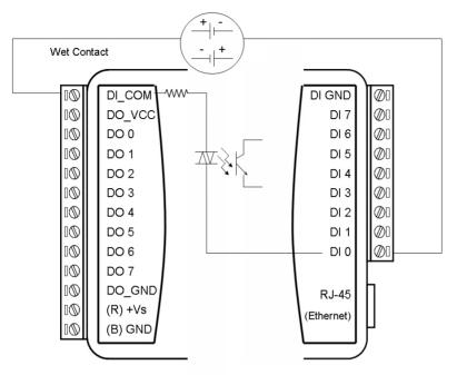
Figure 4.18: ADAM-6052 DI (Wet Contact) Wiring
