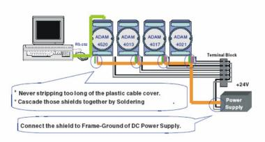
Figure C.11: System Shielding
