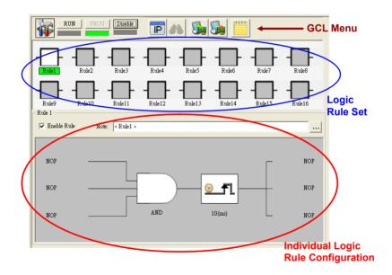
Figure 7.1: GCL Configuration Environment
