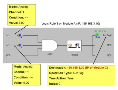
Figure 7.17: Configuration of Logic Rule 1
