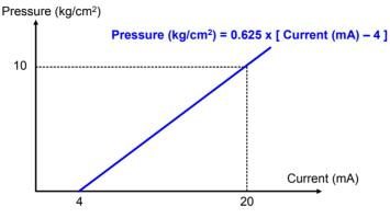
Figure 7.4: Engineer Unit and Current Value
