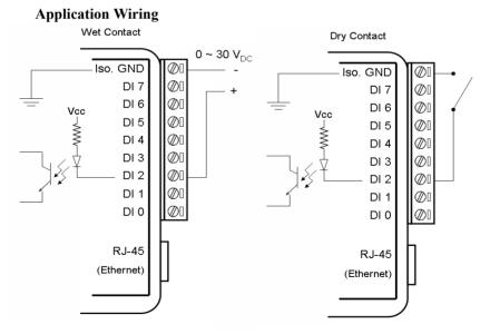
Figure 4.12: ADAM-6050 Digital Input Wiring
