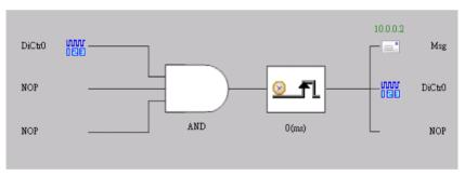
Figure 7.39: GCL Logic for Event Trigger (Only Occurs Once)
