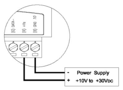
Figure 3.5: ADAM-6000 Module Power Wiring
