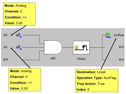
Figure 7.13: Configuration of Logic Rule 1
