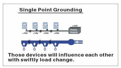
Figure C.7: Single Point Grounding (1)
