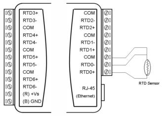
Figure 4.1: ADAM-6015 RTD Input Wiring
