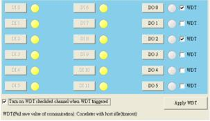
Figure 5.13: Fail Safe Value Configuration
