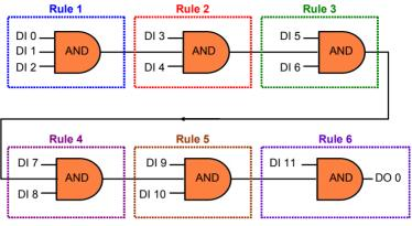
Figure 7.28: GCL Logic for 12 DI to 1 DO
