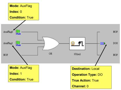
Figure 7.15: Configuration of Logic Rule 3
