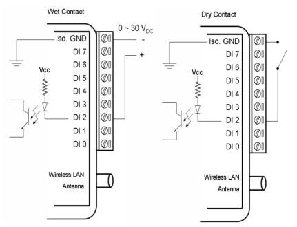
Figure 4.26: ADAM-6051W Digital Input Wiring
