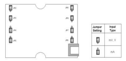
Figure 4.3: ADAM-6017 Analog Input Type Setting
