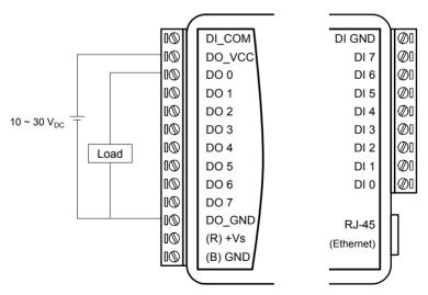
Figure 4.19: ADAM-6052 Digital Output Wiring
