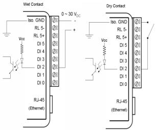
Figure 4.22: ADAM-6066 Digital Input Wiring
