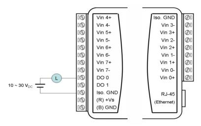
Figure 4.4: ADAM-6017 Digital Output Wiring
