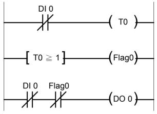
Figure 7.35: Ladder Diagram for Falling Edge
