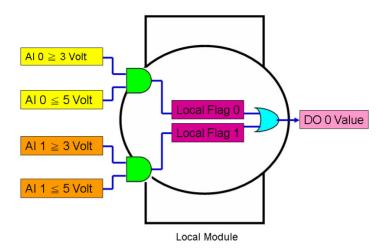
Figure 7.12: Architecture of Local Logic Cascade
