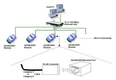
Figure 2.1: Ethernet Terminal and Cable Connection
