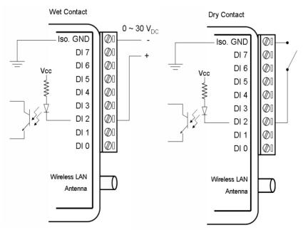
Figure 4.24: ADAM-6050W Digital Input Wiring
