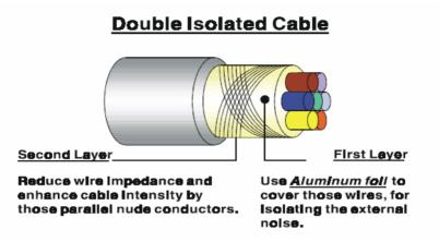
Figure C.10: Double isolated cable
