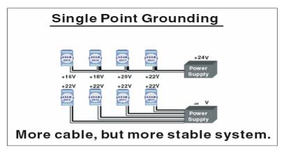
Figure C.8: Single point grounding (2)
