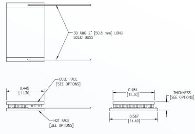
Ceramic Material 96% Alumina Ceramics Solder Construction: 138°C BiSn
