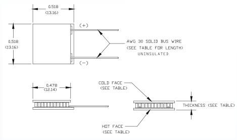
Ceramic Material 96% Alumina Ceramics Solder Construction: 232°C SnSb
