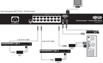
Figure 5.4 NetCommander KVM system connections
