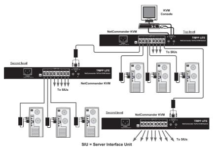
Figure 5.9 Cascading NetCommander KVM Switches
