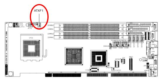
When user would like to use ATX mode, ATXF1 needs to connect to the CN1 on the Advantech backplane to enable the ATX function, 5Vsb.
