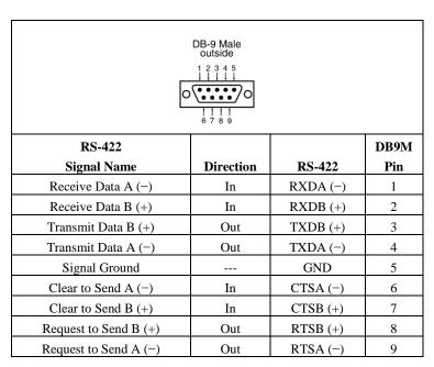
Figure 51. RS-422 Connections in a DB-9 Connector
