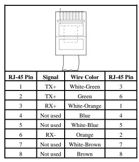
Figure 57. Pin-out for a Crossover Ethernet Cable
