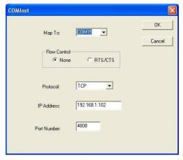
Figure 4. Configuring the Virtual COM Port
