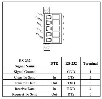
Figure 50. ESR901 Terminal Block Pin-out in RS-232 Mode
