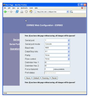
Figure 41. The Web Server Serial Port Properties Page
