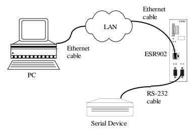
Figure 2. Typical Hardware Setup
