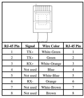
Figure 56. Pin-out for a Standard Ethernet Cable
