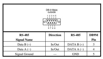
Figure 53. DB-9 Pin-out in RS-485 Mode
