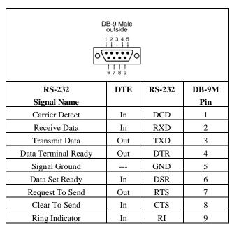
Figure 49. RS-232 Connections in a DB-9 Connector
