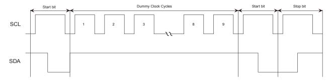
The ATAES132A requires that the clock be pulled low between the Start condition and the Stop condition at the end of the sequence, as illustrated in Figure J-7. It will not reset if this clock transition is omitted. See Appendix J.4, I<sup>2</sup>C Interface Synchronization Procedure for detailed I<sup>2</sup>C interface resynchronization instructions.
