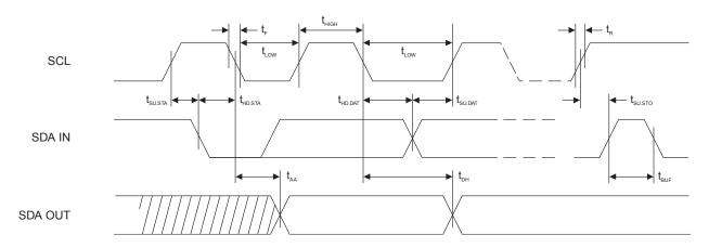
Figure J-10. I<sup>2</sup>C Write Cycle Timing
