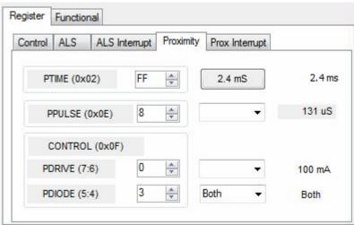
PDIODE – choses the active photodiode(s) for proximity sensing.
