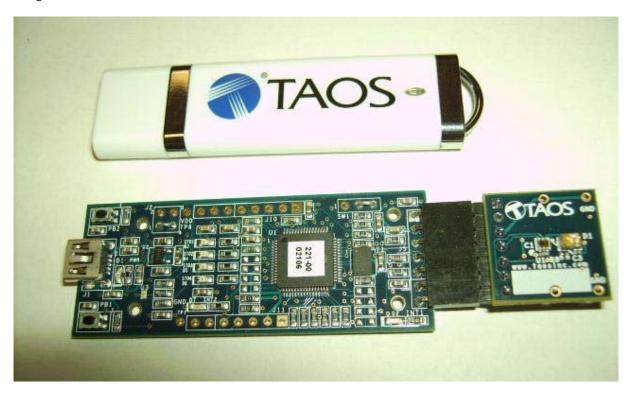
When the USB cable is connected the green LED should light up indicating that power is being received via the USB interface, and the controller board processor is running. If the green LED does not light up check the USB cable connections unplug the USB cable and try again. If after re-try no green LED check the PC for USB error messages. See resources section at end of this document for additional assistance.
