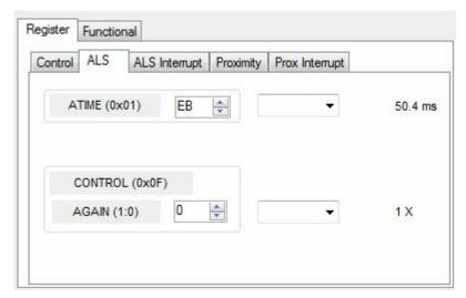
Note: The column on the right is the computed value for ATIME and is always correct. Sometimes the value shown in the list box will be one of the preselected values but it has not been selected. If this happens the number will not be the same as the computed number for WTIME on the Control Sub-Tab. The computed value is the one that is correct. This can be fixed by selecting a preselected value from the list box or by cycling the register value UP/DOWN or DOWN/UP. This will set the list
