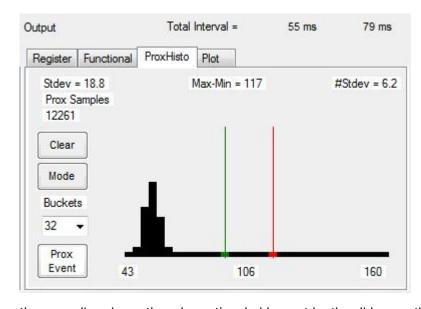
This tab contains a histogram of the recent prox evaluations. It is displayed as a rolling histogram spanning the number of readings in the Test tab of the input.
