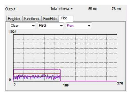
The graph shows all outputs for a static system. The X-axis plots 376 points then rolls over back to 1 on the graph. The Y-axis is set to range 0 to 1024; this range cannot be adjusted. However Multipliers (selected from the list boxes) may be used to scale the display accordingly.
