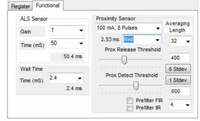
• The "Prox Release Threshold" and "Prox Detect Threshold" sliders allow a threshold (with hysteresis) to be selected to determine when a proximity detection occurs. The thresholds can be set to any value from 1 to 1022. The values selected are shown numerically below the sliders.
