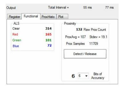
The Prox indication shows the current reading (Raw number) and the rolling average. The average is computed over the number of samples specified on the INPUT/Functional tab.
