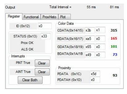
The value of internal registers is displayed on this tab. Register values cannot be set here. To set registers use the Register tab on the input side of the screen.
